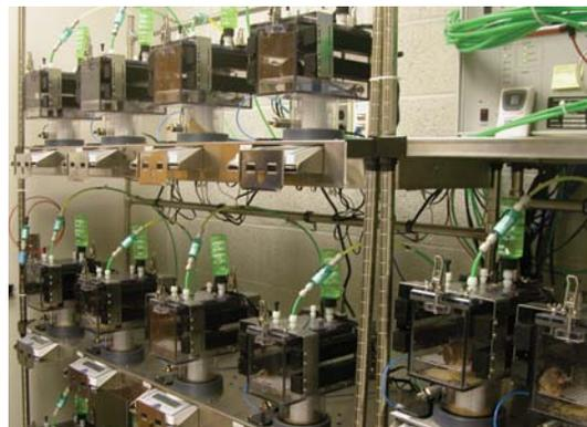
**Figure.** The Healthspan Assessment Laboratory includes a 16-chamber Comprehensive Laboratory Animal Monitoring System (CLAMS) for measurement of respiratory exchange ratio and energy expenditure and simultaneous quantification of habitual physical activity and food intake.
